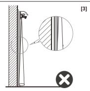
When install it on the door leaf, recommended that the tilt angle of sensor will be ≥15°, ensure laser beam doesn't scan the door leaf, sensor detection will be more stable.
