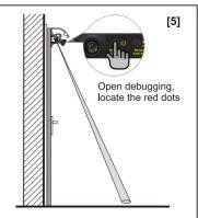
Open the debugging positioning red dots, confirm the general position of the sensing beam(Red dots isn't laser beam, laser beam is invisible light)
